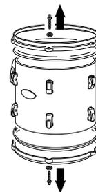
2. Loosen the Allen screws on both sides of the OptiMount and extend the Extension Rods far enough to clear the top and bottom lugs.
