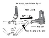
After adjusting the arms tighten the key bolts securely. Failure to do so may cause the drum to fall from the stand.
