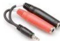
When using a cable or adapter to split the QuNexus CV input port to get 2 mono inputs and 5V power: tip is white (or black), 1st ring is red, and the 2nd ring is yellow. This can vary from cable to cable.
