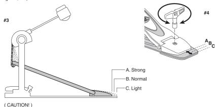
The heel must be flush with the Power Plate, or damage to the pedal may result.
