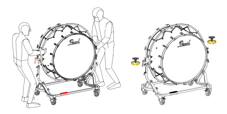
Height Adjustment: With two people, adjust the height of both sides at the same time. Loosen the locking handles, lift to the desired height, and then secure in place with the locking handles.
