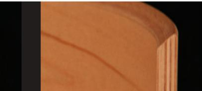
**THICK (8-ply, 10mm and 10-ply, 12.5mm)** Maximum projection and quick decay.
