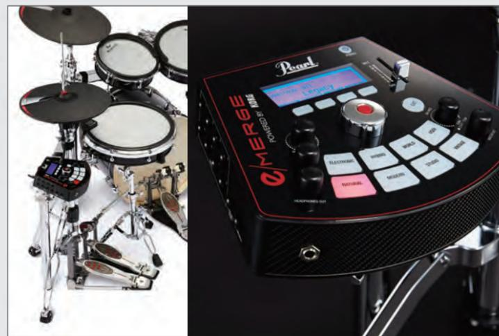
**WAVE TRIGGER TECHNOLOGY** This ultra-fast and highly sensitive technology partially based upon KORG's groundbreaking Wave Drum allows even your stick choice to make a discernible difference in the sound of your drum.
